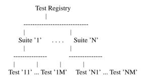
Individual test cases are packaged into suites, which are registered with the active test registry. Suites can have setup and teardown functions which are automatically called before and after running the suite's tests. All suites/tests in the registry may be run using a single function call, or selected suites or tests can be run.
